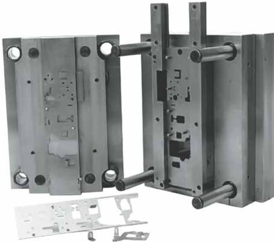
Calmax用在冲压和穿孔的级进模
